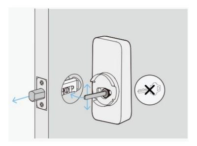
Place assembly and torque blade through the deadbolt slot and guide connection cables under the deadbolt as shown.
