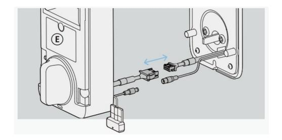
Click the rounded antenna connectors in to the built-in clip.
