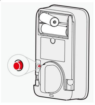
With the door open and the deadbolt fully extended, insert the battery.
