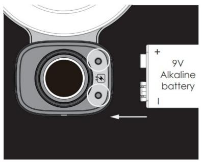
Hold a 9V alkaline battery against the contact points located at the bottom front side of the lock hold to activate the fingerprint reader and scan a registered fingerprint to unlock. Once unlocked, replace batteries immediately.
