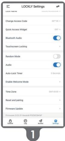
Enable this feature through the Lockly App. Go to > **Settings > Enable Welcome Mode**, then slide button to enable and set the specific time you require your door unlocked
