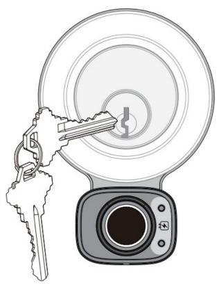
Lockly Flex Touch is designed to convert your existing deadbolt to a smart lock and keep your existing physical keys. To unlock your lock using the your physical key, insert key and turn clockwise or counterclockwise to lock or unlock the door.
