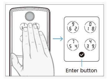
Ten consecutive wrong attempts will put Lockly in "Safe Mode". You may toggle between two types of keypad displays to enter your Access Code. The fixed digit version and the PIN Genie version (Recommended). Press and hold the Enter Button for 3 seconds to toggle back and forth between the two keypads.(Sample display shown only)
