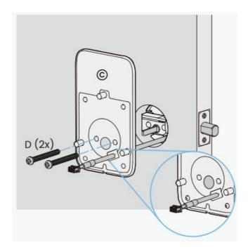
Using the key, check that the deadbolt locks and unlocks smoothly. If the key does not turn the deadbolt, revisit the steps above and ensure the plate is properly aligned with the exterior assembly.
