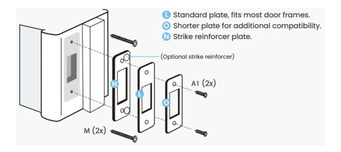
Due to variations in door and frame designs, you may need to adjust the strike plate to ensure smooth deadbolt operation. This is crucial. If the deadbolt binds or catches, the lock will beep rapidly, indicating it cannot close due to misalignment or excessive rubbing. Refer to the included Strike Plate Installation Locator Kit for help.
