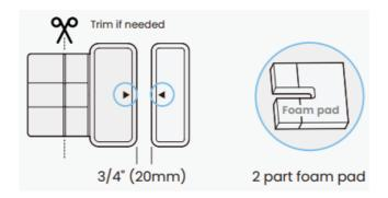
Align the arrows on each sensor, ensuring the gap is less than 3/4". Sensors must be as level with each other as possible. Use adhesive foam pads to adjust the door wired sensor's height if needed.
