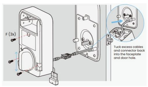
Align outer thumbturn and torque blade shaft, make sure both are in the vertical position. Carefully tuck cables and connector back into the faceplate and door hole under the deadbolt. Be careful not to force or pinch the cables.
