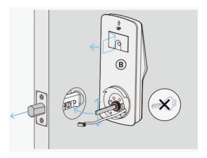
Place assembly and torque blade through the deadbolt slot and guide connection cables under the deadbolt as shown.
