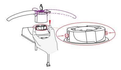
3.3 Rotate the handle 180 degrees to the other side of the lock. Using your fingers, press the two pins located on the left and right side of the lock to insert the handle back onto the lock.
