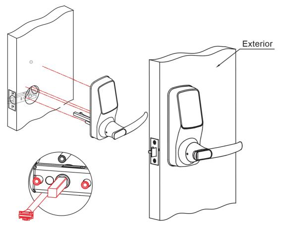
5.3 Pass the square rod (Part C) through the center of the lockset, and the round rods through the sides in their respective holes. The cable should run underneath the lockset.
