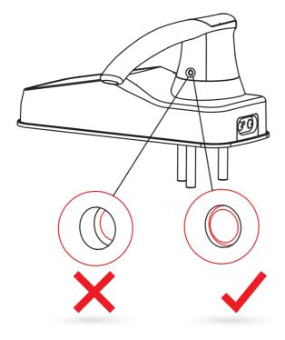
3.4 Confirm that your installation was complete by checking if the pins are flush against the handle, and has popped out. Adjust the handle accordingly to make sure the pins are fully decompressed and sits flush against the surface.
