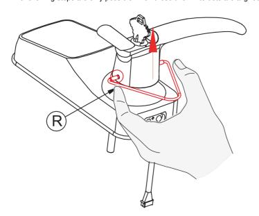
3.2 Use the provided Clamping tool (R) to push in the two metal pins at the base of the lock handle, located at the 3 o'clock and 9 o'clock positions, and remove the handle once the pins are compressed.
