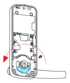
3.6 Remove the screw by turning counterclockwise and rotate the handle 180° in the direction of the arrow as shown.
