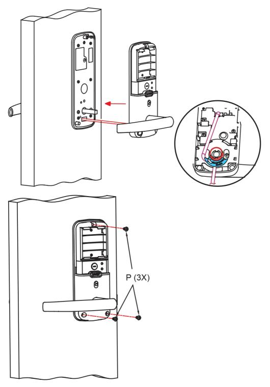
6.7 Once the Interior lock is flush against the mounting plate, secure the lock to the plate by screwing clockwise by using supplied screws (Part P).
