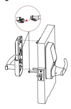
6.5 Plug the cable that is coming through the door into the interior lock. Make sure you match the direction of the plug correctly and matching the red side of the plug with the red side on the lock.
