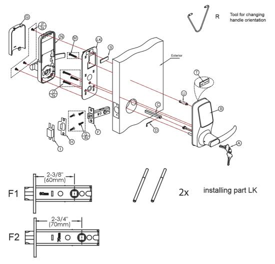
Measure distance between the center of the hole to the edge of the door: Use F1 if 2-3/8"(60mm) or F2 if 2-3/4"(70mm)
