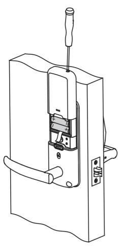
6.8 Insert 4 AA batteries into the lock by matching the positive (+) and negative (-) orientation markings on the batteries to the battery chamber. Secure the battery cover by sliding the cover over the lock and turning the screw clockwise on top until tight.
