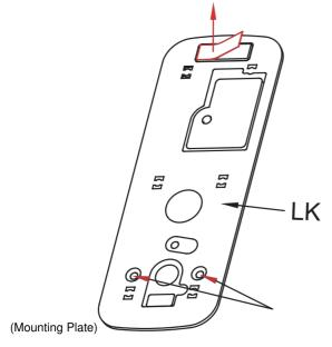
Positioning rods slide through these holes.
