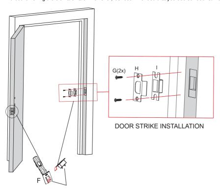
Make sure the slanted side of Part F1/F2 is closing against the slanted part of Part H before fixing it on to door frame.
