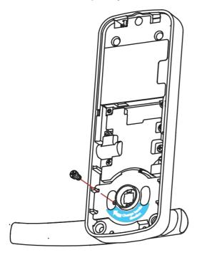
3.7 Securely screw clockwise as shown to complete your handle orientation change.
