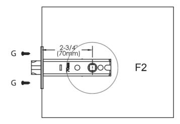
2.2 Install the lockset with the slanted side of the latch facing towards the closing direction.
