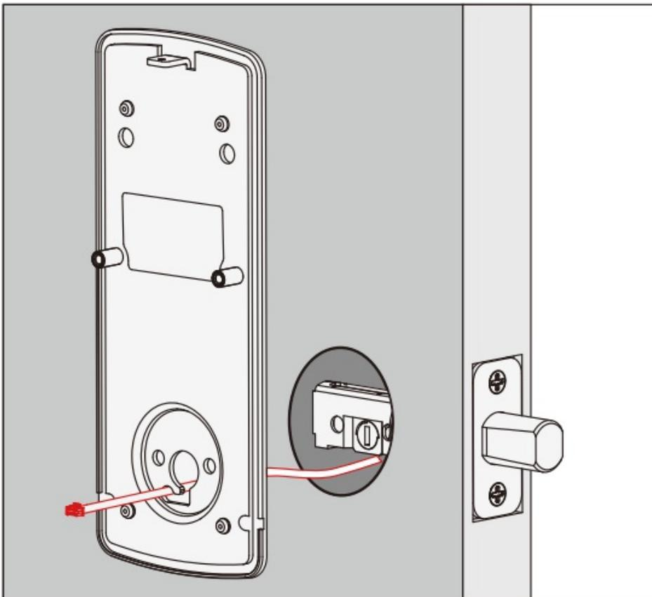
3. Insert, tighten by hand 2 screws located on the left and right of the blade. Check alignment and tighten with screwdriver until mounting plate is securely placed on door.
