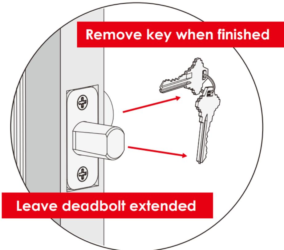
**IMPORTANT:** when finished, leave the deadbolt extended and remove the key before proceeding to the next step.
