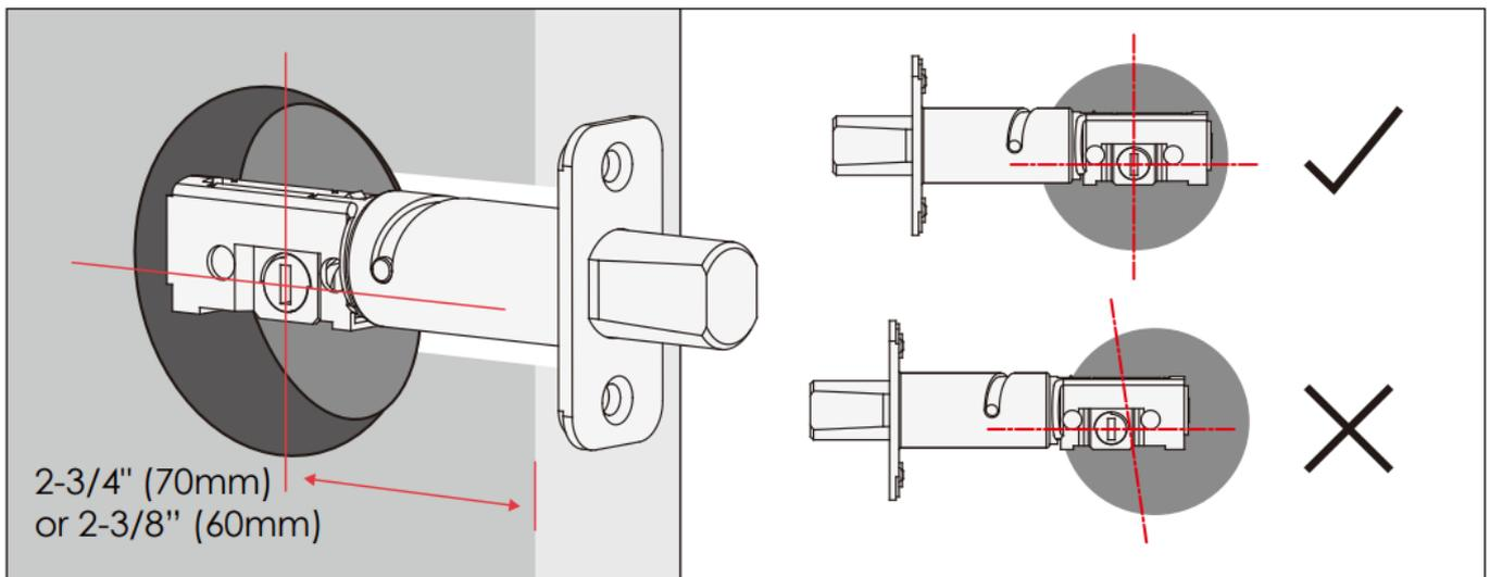
The deadbolt comes set to 2-3/4" (70mm). Adjust length to 2-3/8" (60mm) if necessary. (wear gloves to protect from possible pinching).
