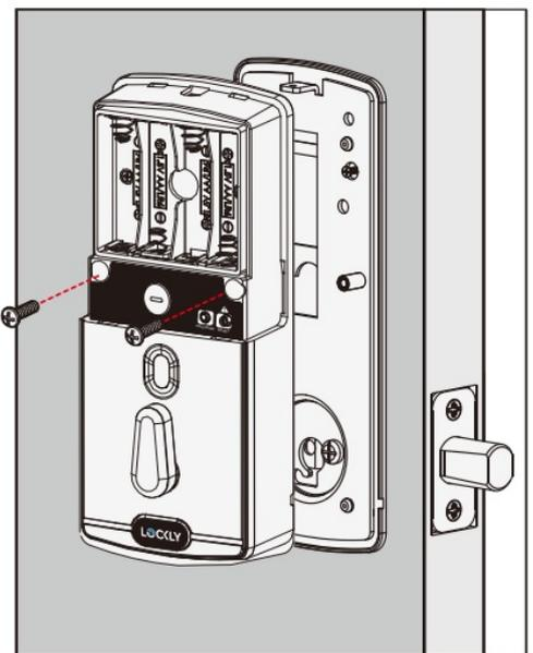
Before placing the interior assembly onto the mounting plate, ensure the thumb turn is vertical.
