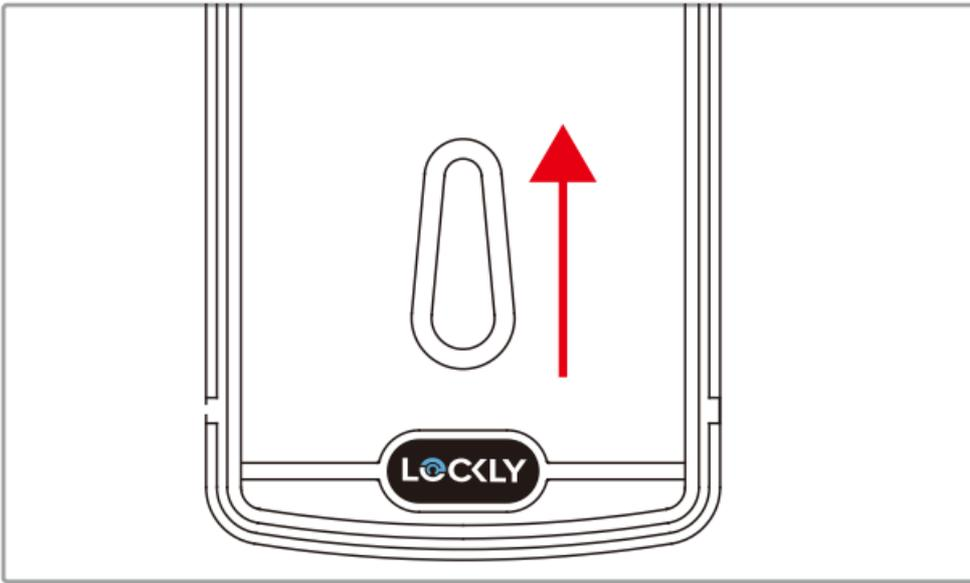
Place the interior assembly against the mounting plate and make sure the torque blade is inserted to the thumb turn shaft.
