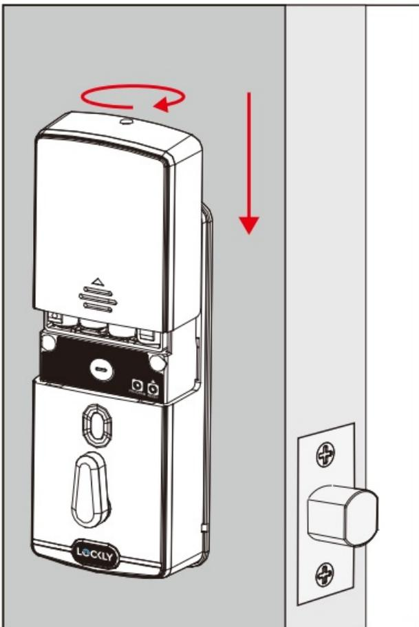
4. Once self-check is complete, install the battery cover (H) and secure with screw on top (do not over tighten).
