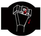
**NOTE:** If you need to disconnect the cable, make sure to press the snap tab to release the plug before carefully pulling it out. Do not force, as this may result in damaging the lock.
