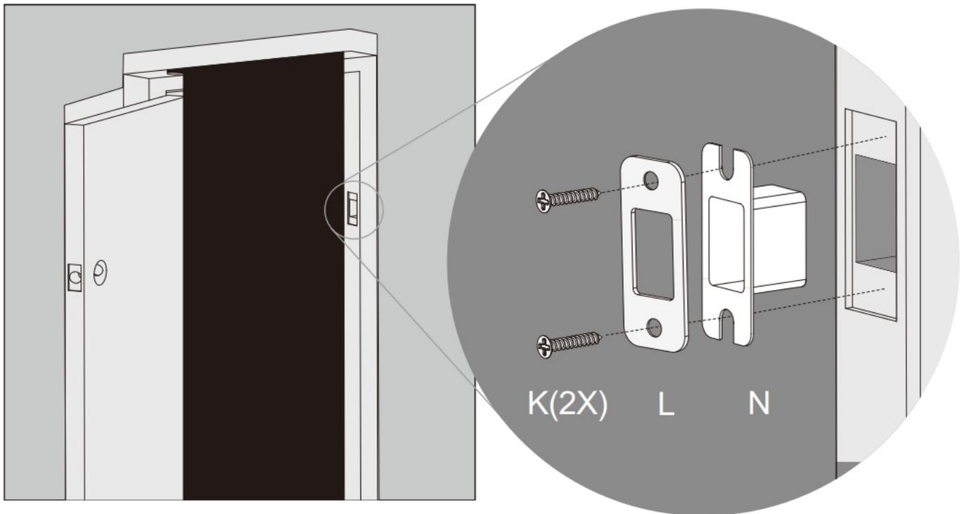
**IMPORTANT:** Because doors and frames vary in design, it may be necessary to make slight adjustments to your strike plate and/or dust box in order to ensure smooth deadbolt operation. This is
