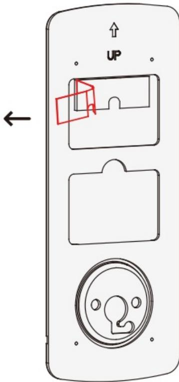
2. Align and secure mounting plate with adhesive strips. Guide connection cable through and secure to the lower left notched hole.
