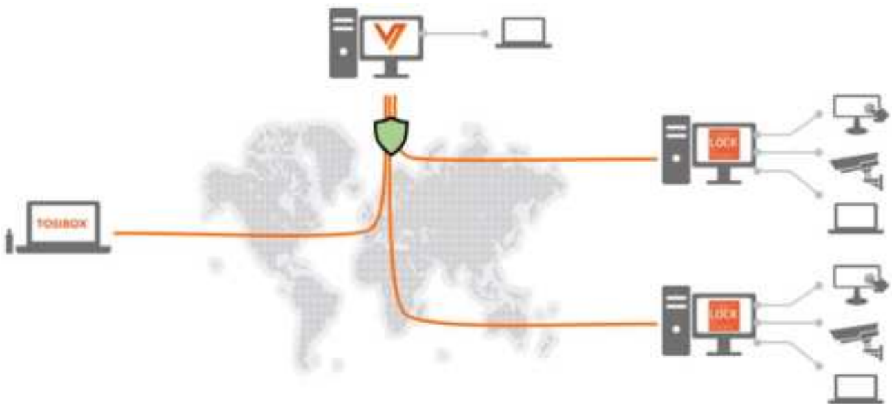
Figure 3: Connectivity from TOSIBOX® Key Client to devices behind TOSIBOX® Lock for Container via TOSIBOX® Virtual Central Lock
