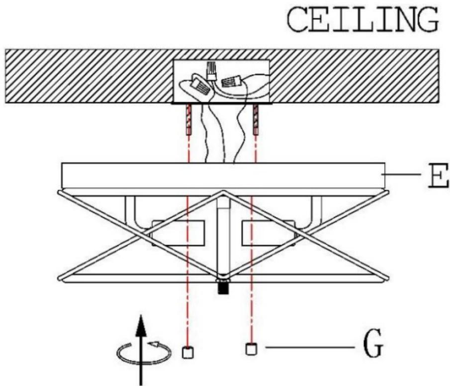
**Note:** canopy (E) should be snug against the ceiling and knob nuts (G). If not, adjust the threaded length on the mounting plate assembly (C):
