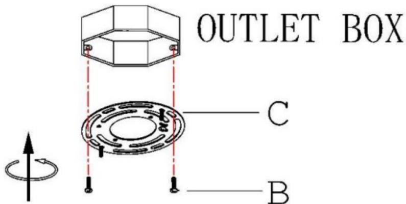
**NOTE:** The side of the mounting plate (C) marked “GND” must face out.
