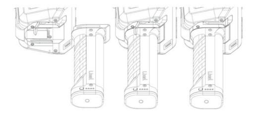
Note: An unsecured battery may cause the device to slip.
