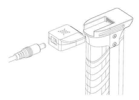
Use the standard charging cable and connect the charging adapter to the battery to charge the battery. Charging time: about 2 hours. During the charging process, the indicator light will show the current electric quantity. Please refer to the following table for details.
