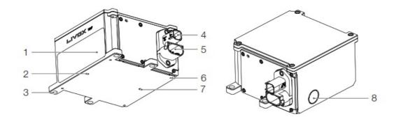
Installation and Connection Effective FOV Range HAP (T1) has a FOV of 120° (horizontal) x 25° (vertical) as shown below. When mounting HAP (T1), make sure that the FOV is not blocked by any objects. Visit <a href="https://www.livoxtech.com/hap">www.livoxtech.com/hap</a> to download the 3D models of HAP (T1) and its FOV.
