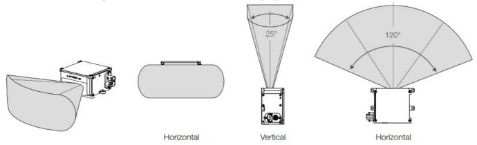
Note that the effective detecting distance of HAP (T1) varies based on where the object is within the FOV. The closer to the edge of the FOV, the shorter the effective detecting distance is. The closer to the center of the FOV, the further the effective detecting distance. Refer to the diagrams below.
