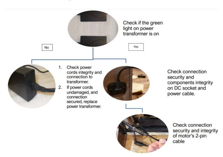
For dual-power recliners, please check the connection and integrity of the Y-Cable splitter.
