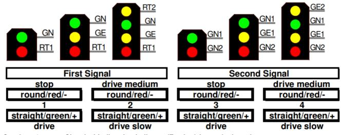
2. One 2- to 4-aspect Signal with direction indicator (Feather) for each clamp bar:
