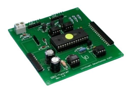
Master-Module for Decoder for Switchboard Lights from the Digital-Professional-Series!
