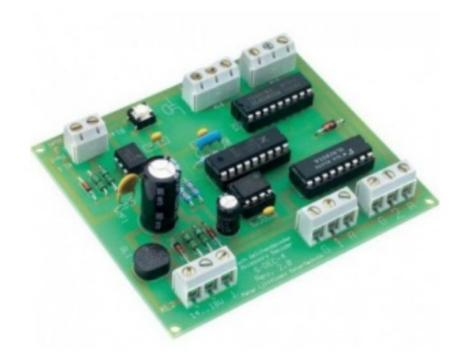
Master-Module for Decoder for Switchboard Lights from the Digital-Professional-Series ! GBS-Master-MM-F Part-No.: 050322
