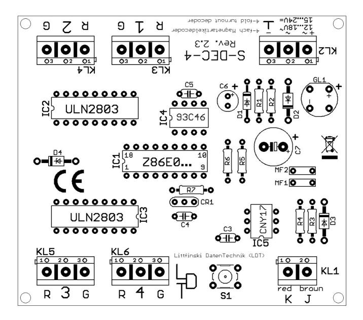
Now connect turnouts, signals, uncoupling tracks or the permanent power switch units [DSU] to the 3-pole clamps marked 1 to 4.
