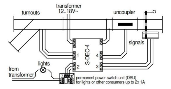
With our permanent power switch unit [DSU], which is equipped with a bi-stable relay, it is possible to switch lights or other consumers up to 2x 1A digital on or off.
