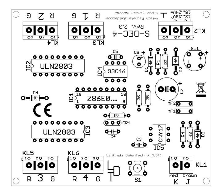
Now connect turnouts, signals, uncoupling tracks or the permanent power switch units [DSU] to the 3-pole clamps marked 1 to 4.
