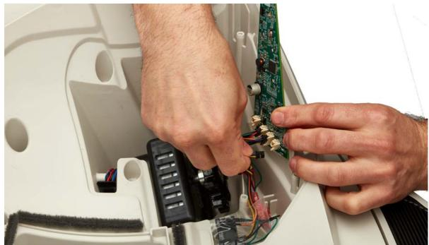
9. Before installing the new circuit board, ensure that the motor sits flush in the motor cavity and that no wires are in the way of the motor's gear.
