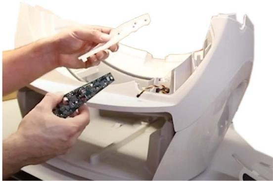
11. Install the rubber circuit board cover over the new circuit board. Make sure that it is securely fitted along all of the edges.
