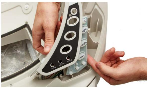
15. Once all the connections are secured, replace the circuit board cover and secure it with the 5 screws.
