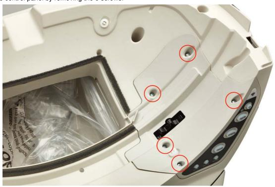
7. Carefully remove the circuit board cover; take care not to lose any of the screws.
