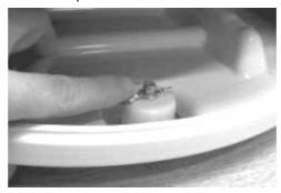
• Locate the Cat Sensor Switch directly under the waste drawer at the front of the base.
