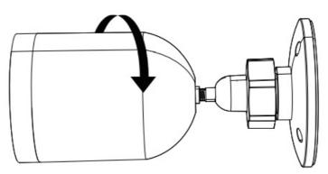
4. Adjust the camera angle to get the best field of view. And secure the camera by turning the bracket clockwise.
