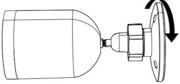
2. Drill holes in accordance with the installation holes on the bracket and Install the bracket with screws included in the package.
