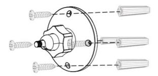
3. Screw the camera to the bracket.
