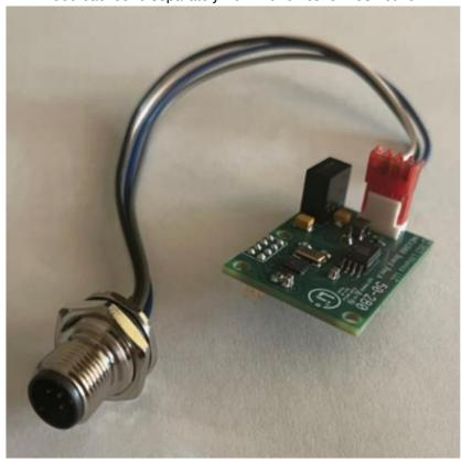
NMEA2000 add-on board was developed, which can be installed inside the NeverDie V9 External BMS as an optional feature. Once installed, the BMS firmware automatically detects it and starts sending NMEA2000 messages to this CAN interface.
