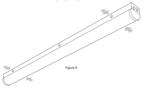
2. Locate the surface mounting holes. Raise empty fixture into place and drive two mounting screws directly into the mounting surface/anchors. **See figure B.**
