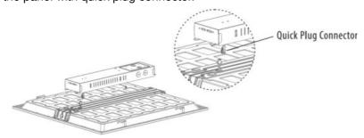
2. Push the driver into the slot position.
