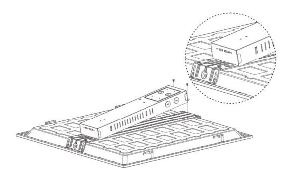
2. Push the driver into the slot position.
