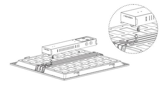
1. Connect the driver to the panel with quick plug connector.
