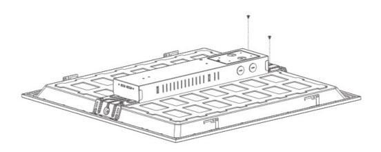
3. Lock the driver box on the bracket by screws.
