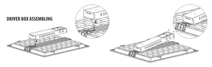
3. Lock the driver box on the bracket by screws.
