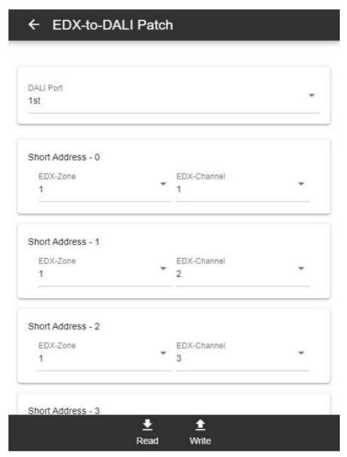
• It is able to determine the mapping between the EDX zone/channels and the DALI short address.
