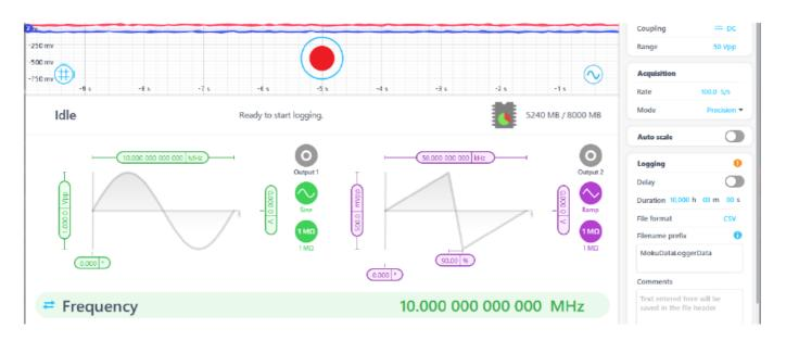
The Moku:Go Data Logger has a built-in Waveform Generator capable of generating basic waveforms on the two output channels. Find detailed instructions for the Waveform Generator instrument in the Moku:Go Waveform Generator manual.
