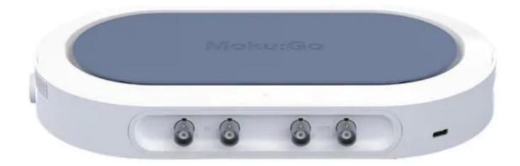
**The Moku:** Go Data Logger instrument records time series voltages from one or two channels at rates from 10 samples per second up to 1 MSa/s. Log data to the onboard storage or stream directly to the computer using the Moku API. The Moku:Go Data Logger also includes a two-channel embedded waveform generator.
