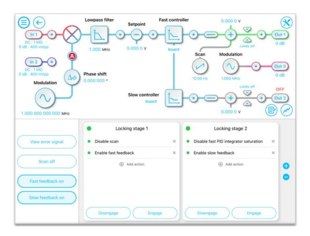
The lower half is readily set to display one of three parameter control panels: locking stages, Oscilloscope, and Data Logger.
