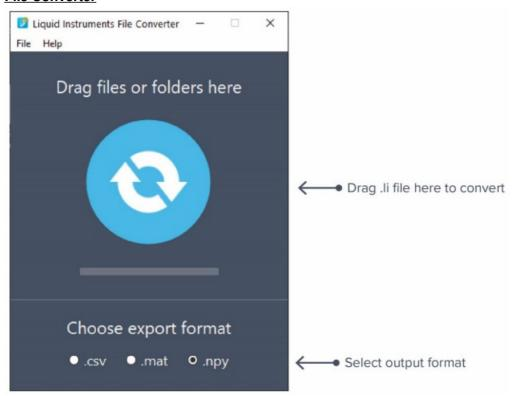
The converted file is saved in the same folder as the original file. Liquid Instruments File Converter has the following menu options:
