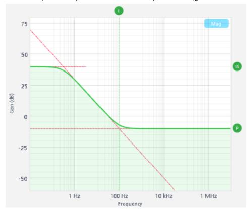
The green/purple solid curve represents the active response curve for PID Controller 1 and 2, respectively. The green/purple dashed vertical lines (04) represent the cursors crossover frequencies, and/or unity gain frequencies for PID Controller 1 and 2, respectively.
