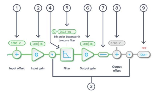
The two independent, real-time configurable digital IIR filter paths follow the control matrix in the block diagram, represented in green and purple for filters 1 and 2, respectively.
