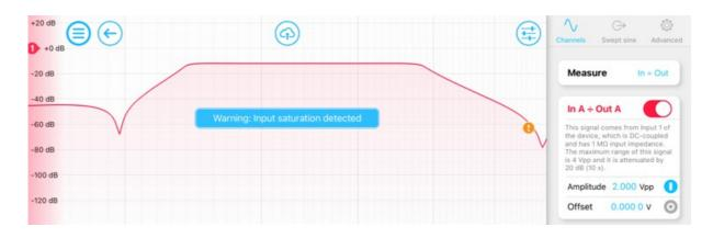
Clicking the orange exclamation icon on the right-hand side of the graph will provide additional information regarding which frequencies are saturated and possible solutions, including enabling dynamic amplitude mode.
