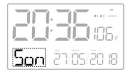
5. Short press " ♣ 1 " button again, and "L01" begins to flash. Press " ▲ "or" ▼ " button to adjust the volume among L01, L02, L03
