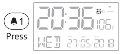
2. Long press " • 1" button to enter Alarm 1 setting with Hour digit flashing. Press " • " or " • " button to increase or decrease by one digit, and long press to quickly adjust.
