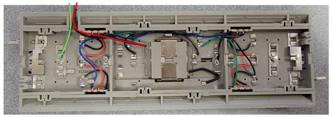
• Step 5. Connected the 2 wires from the Operating Track section to the ASC2.
