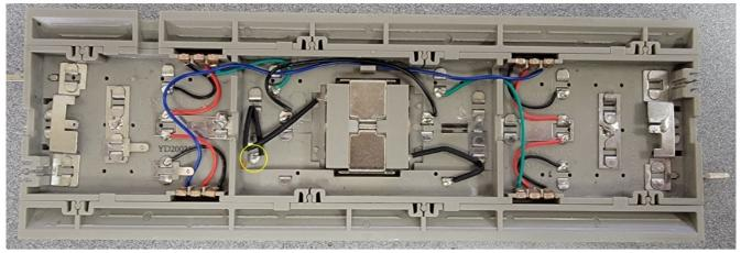
• Step 3. Solder ground wire from where blue quick connect was to the adjoining outside rail as shown below in light blue.
