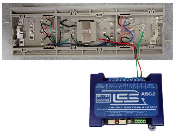
• Step 6. Connected the "COMM" terminal on the ASC2 to either accessory power or track center rail.
