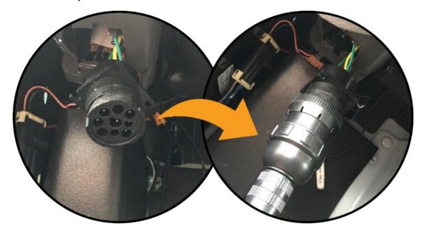
3. Turn on the ignition, and verify green and orange lights on the device.
