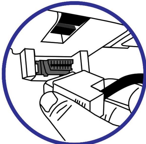
3. Turn on the ignition, and verify green and orange lights on the device.
