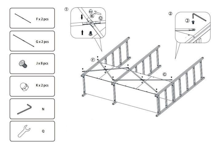
Fasten x-bar reinforcement by screws.
