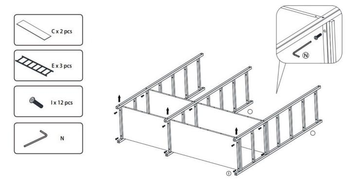
Keep the screws in the same direction at its installation
