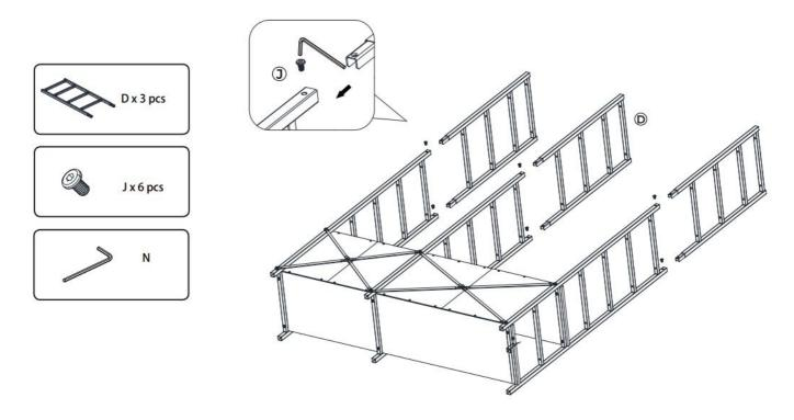
Insert the top brackets into the bottom brackets then fasten with screws.
