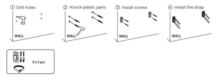
Install the furniture anchors by drilling holes on the wall and the leveler feet based on needs.
