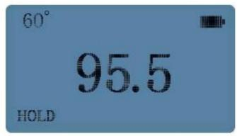
(2) QC Mode If the instrument is set to QC mode, remove the calibration holder after calibration, place the measuring port of the instrument on the surface of the object to measure, short press the button to measure, the instrument will judge whether the measured value is qualified. The upper and lower limits could be set by PC software. For specific operations, please refer to the "Gloss Meter Software Operation Manual".
