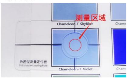
• Place the meter on the positioning hole
