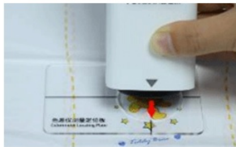
Place the meter on the positioning hole
