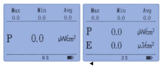
• In the measurement mode, if the backlight is off, press the Hold button to light the backlight; if the backlight is already lit, short press the Hold button, and the "HOLD" icon will be displayed in the lower-left corner of the interface. All data will be held on the LCD, and the current data will be recorded.
