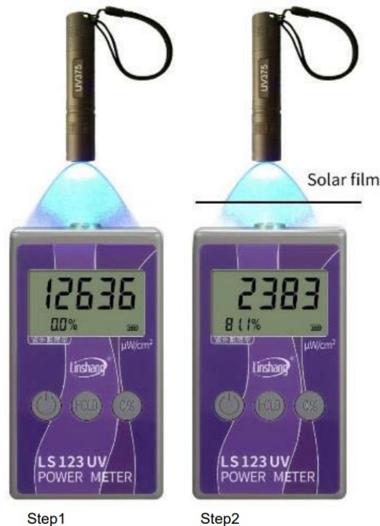
Figure1: Measuring the UV rejection rate of solar film
