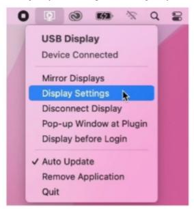
3. Mirror Displays: Click here to change mode between Mirror Display or Extended Display.
