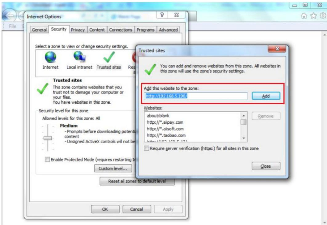
**Step4:** Enter the IP address. After logging on to web GUI successfully, the user is allowed to view live video.
