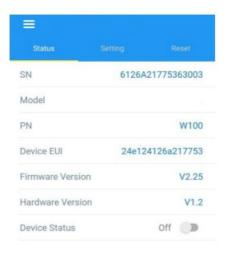
3. Change the on/off status or parameters, then attach the smartphone with NFC area to the device until the APP shows a successful prompt.
