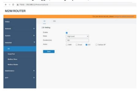
You can configure DO to be low by default and Duration: 1000\*10ms. At this time, the LED is off.
