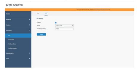
When DI-IN receives a switch signal, it will be linked to DO. After DO is output, the LED will turn on for 10s, and then turn off.
