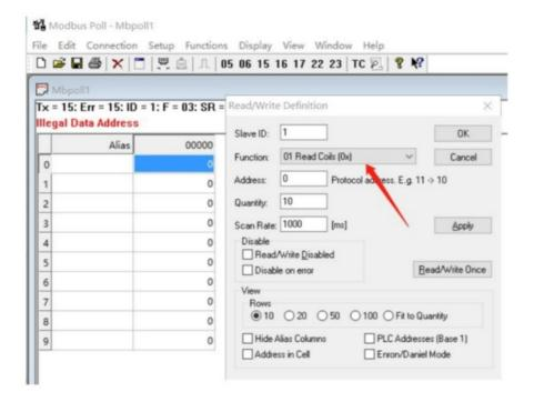
**d**. View the current DO port status according to the output address bit set on the router (DI port needs to be read with function code 02).
