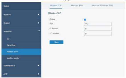
**b**. Open the Modbus Poll tool, select Modbus TCP/IP when connecting, fill in the router IP and port (default 502) and click ok to connect.
