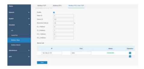
**c**. The DO status can be modified by issuing a command on the server side, and the router will reply the same command when the sending is successful.
