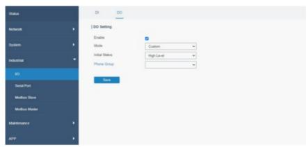
Message content: set **do1 low,20** //20 means the time of DO output low level, the unit is second; when the time is set to 0, it means it remains constant When DO wants to stay low, send set **do1 low,0** Send when DO is to be kept high: **set do1 high,0** Query the current DO status: **do information**
