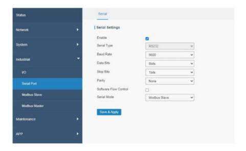
c. Enable Modbus RTU function and select the corresponding serial port.
