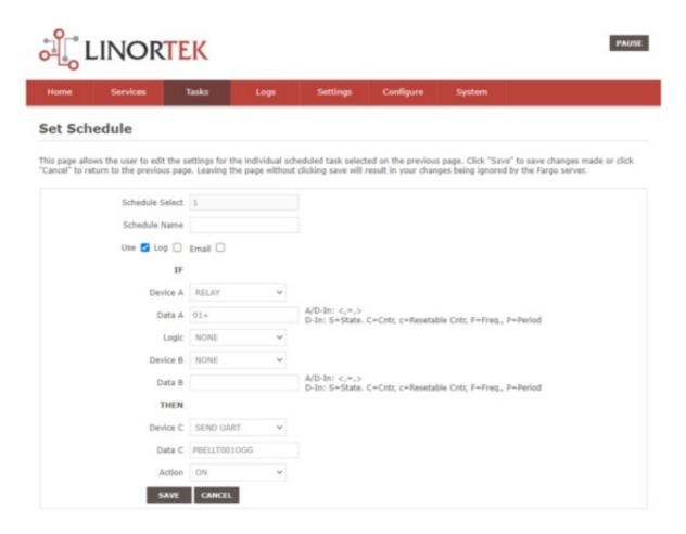
Now you have assigned a tone to relay 1. To test the sound manually, go to **Services – Relays** page, click the red dot under State column, when it turns green, the assigned tone should be played through your speakers.
