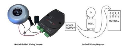
There are 2 relay (bell) outputs (Dry Contact, 1-Form-A relay 48VAC@8A Max) for the Netbell-2 and are simply numbered OUTPUTS "1" and "2". These relays are Normally Open and you can use it to control up to 2 bells directly.
