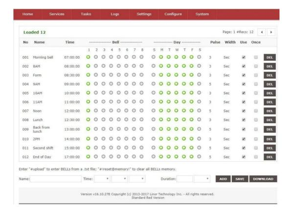
Each Linortek web relay controller includes a remote function that can deliver a signal from a master controller to remote slave controllers in multiple locations. To build a MasterSlave system, follow the steps below.
