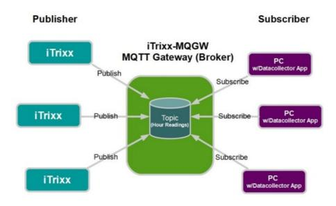
In our example, when we port the gateway to the Internet, we have a new IP address for the gateway (98.25.185.186), the port number stays the same (1883). Connect iTrixx to the gateway new IP address: On Telnet, type in the following commands:
