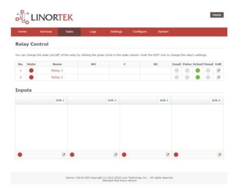
The State LED shows whether the relay is on or off indicated by GREEN and RED respectively. This icon is clickable to manually control the corresponding relay. Each relay can have a Name as well as identifiers for the Normally Open, Common and Normally Closed connections.
