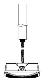
2. Screw the fixture to the 3/4" NPT stem.
